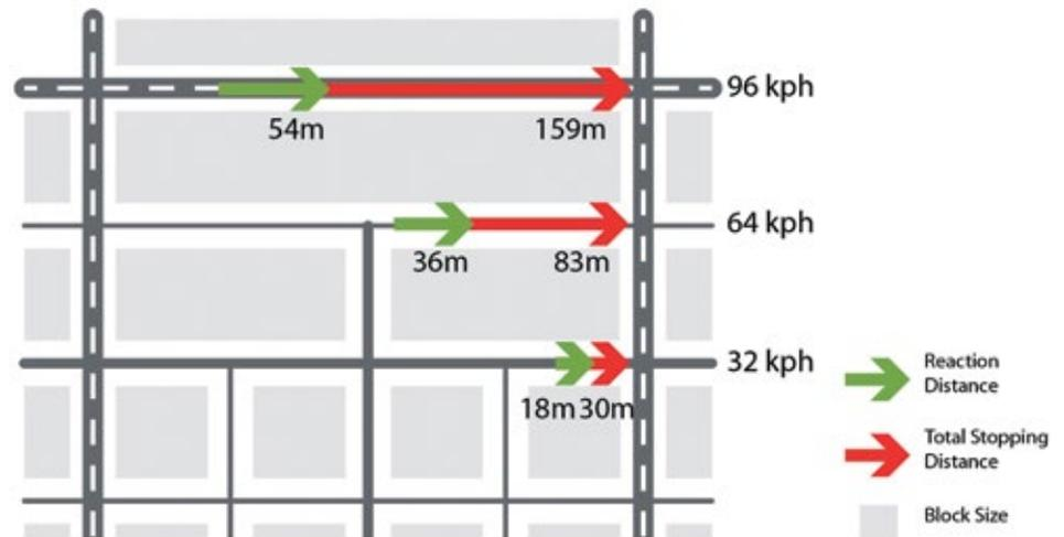
Note: Assumes 2 seconds reaction time and vehicle deceleration rate of 3.4 m/s<sup>2</sup>.
