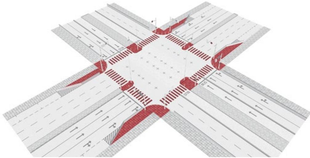
Providing curb extensions and median refuges decrease crossing distance and reduce exposure to moving vehicle traffic.
